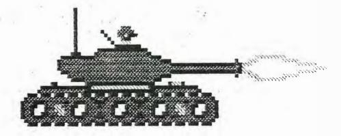
The routine does require a little additional comment. Each poke puts out a column of 8 dot positions some of which may be blank. If the number poked is expressed in binary, the dot positions that are printed correspond to the one bits with the low-order bit corresponding to the lowest dot position. The top 4 dots are in one pixel and the other 4 dots are in the pixel immediately beneath it. Six adjacent columns are used to print the pair of pixels.
